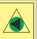
104.287 MM Remote control for bilge pump(s)
