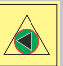
104.288 MM Remote control for emergency bilge pump
