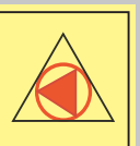
104.286 MM Remote control for emergency fire pump or fire pump supplied by the emergency source of power
